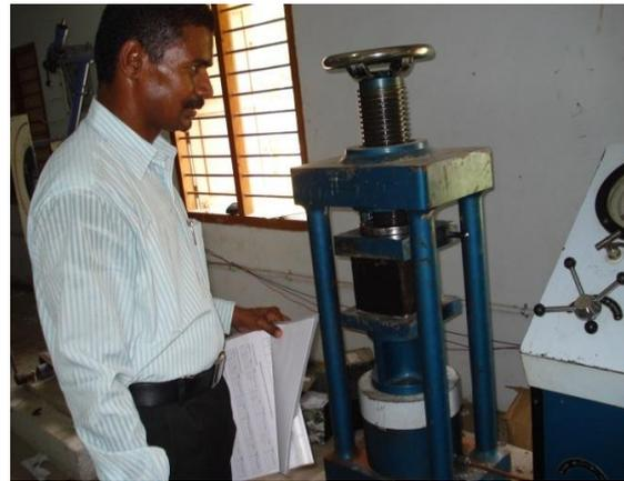
Fig.3 Compressive strength testing
